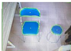
Figure 1. The drone detects landing platforms by their color and shape
