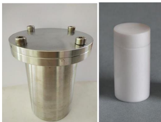
Figure 2. Autoclave Teflon-lined (PTFE) react in hydrothermal reaction
