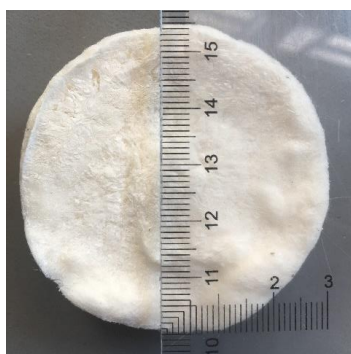
Fig.1: Cotton/pineapple fiber aerogel
