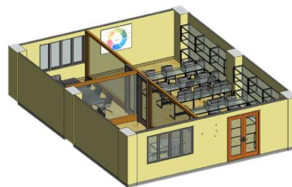
Fig.2: From point cloud model to BIM model of Office
