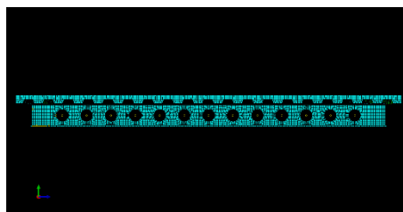
Fig.3 Perforated beam modelled in ABAQUS
