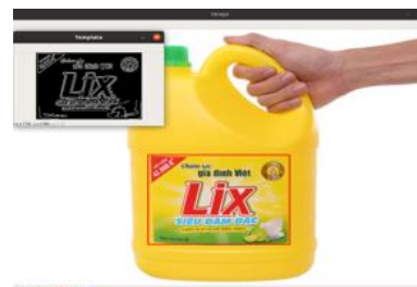
Fig.2: Label detection using template matching
