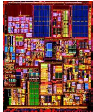
2002 – Intel Pentium 4 2.4GHz – 0.13\mu 55B components 4 km interconnects
