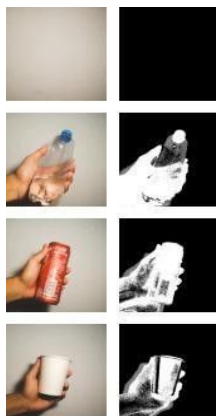
Figure 3. The changes of the mask when a moving object is in front of the camera. The moving object is considered the foreground (white pixels), and the remaining area is the background (black pixels).
