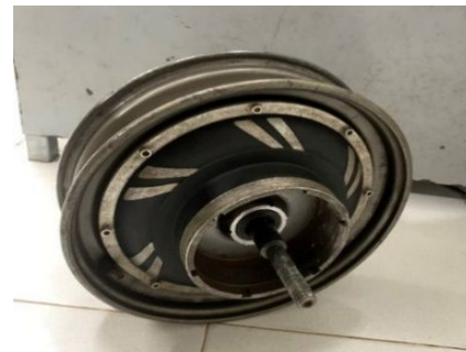
Figure 1. The ZXDCM1208 in-wheel motor
