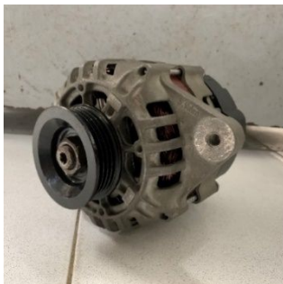
Figure 3. The Valeo SG9S116 alternator
